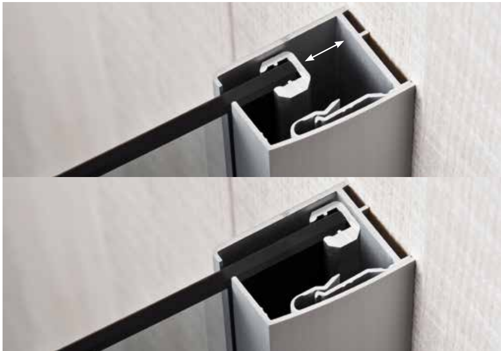
princess 4000 - Whether the glass thickness is 6 mm or 8 mm, under the covers hides the adjustment range of 25 mm.
